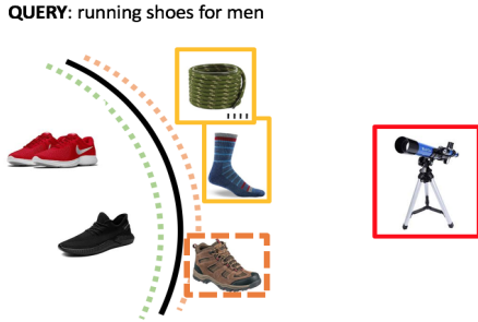
Figure 1: (Best seen in color) The query is running shoes for men . The solid black line illustrates the classification boundary, and each dotted line is a small margin around the boundary. Samples to the left of the boundary are matched. To the right are mismatches, such as socks and shoelaces (orange boxes). To the extreme right is a telescope, which is an easy-to-classify example (red box). Close to the classification boundary is a hiking shoe (orange dotted box) which is a hard-to-classify positive. We want to train a generator that can learn to generate such hard samples.
