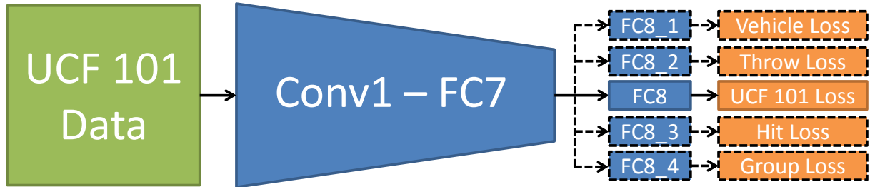
Figure 1: Multitask learning layout: the orange shapes represent loss functions, the blue shapes represent the network, and the green shape represents the input data. Sections outlined with dotted lines denote the additional multitask learning components.
