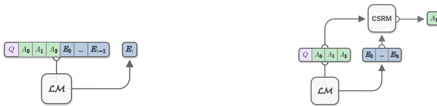
(a) One time-step of training a CAGE language model to generate explanations from CoS-E. It is conditioned on the question tokens Q concatenated with the answer choice tokens A_1, A_2, A_3 and previously generated tokens E_1, \dots, E_{i-1} . It is trained to generate token E_i . (b) A trained CAGE language model is used to generate explanations for a downstream commonsense reasoning model (CSR), which itself predicts one of the answer choices.
