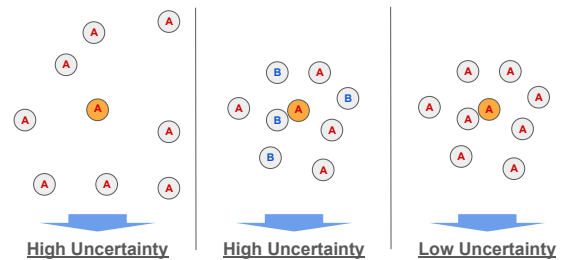
Figure 1: Illustrations of k NN-UE behavior. The orange circle indicates predicted data instances and other circles indicate training data instances. k NN-UE gives high uncertainty when the predicted query representation is far from examples obtained from the k NN search (left) and the predicted label is different from the labels of neighbors (center). k NN-UE outputs low uncertainty only when the query representation is close to neighbors and the labels of neighbors contain many of the model’s predicted label (right).
