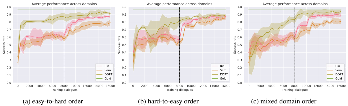
Figure 7: Training the three architectures Bin, Sem and DDPT using CLEAR on three different domain orders, each with 5 different seeds. Each model is evaluated every 500 training dialogues on 100 dialogues per domain. The plots show the success rate, where performance is averaged over domains. The vertical line at 8000 dialogues indicates the start of cycle 2.
