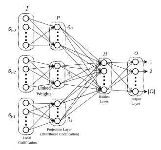
Figure 1: Architecture of the continuous space NN LM during training. The input words are  $s_{i-n+1}, \ldots, s_{i-1}$  (in this example, the input words are  $s_{i-3}, s_{i-2}$ , and  $s_{i-1}$  for a 4-gram). *I*, *P*, *H*, and *O* are the input, projection, hidden, and output layer, respectively, of the MLP.
