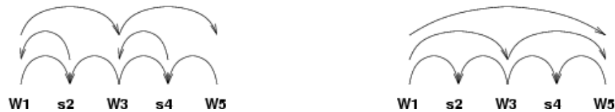
Figure 1: Two FlexGram models where W represents a stem, s represents a suffix, and the arrows represent dependencies. The left model has stem offsets [+1,-2] and suffix offsets [+1,-1] and cannot be used as a directed graphical model because of the cycles. The right model has stem offsets [-4,-2] and suffix offsets [+1,-1] and is the best order-3 FlexGram model for Turkish.
