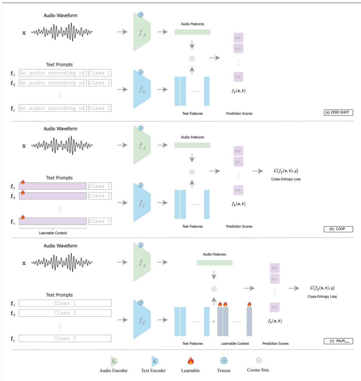
Figure 3: Overview of Zero-Shot, COOP, PALM (a) Zero-Shot inference involves matching the embedding of the audio waveform with the embeddings of text prompts for each class. The class with the highest matching score is then assigned to the audio. (b) COOP (Zhou et al., 2022b) avoids using handcrafted text prompts by learning the context of text prompts in the token embedding space. It optimizes the input space of the text encoder to enhance classification performance. (c) PALM requires only class names at the input of text encoder and it optimizes the feature space by adding learnable context embeddings to text feature vectors. PALM not only outperforms COOP (see Table 2), but it is also more computationally efficient since it does not require gradients to flow through the text encoder, unlike COOP.
