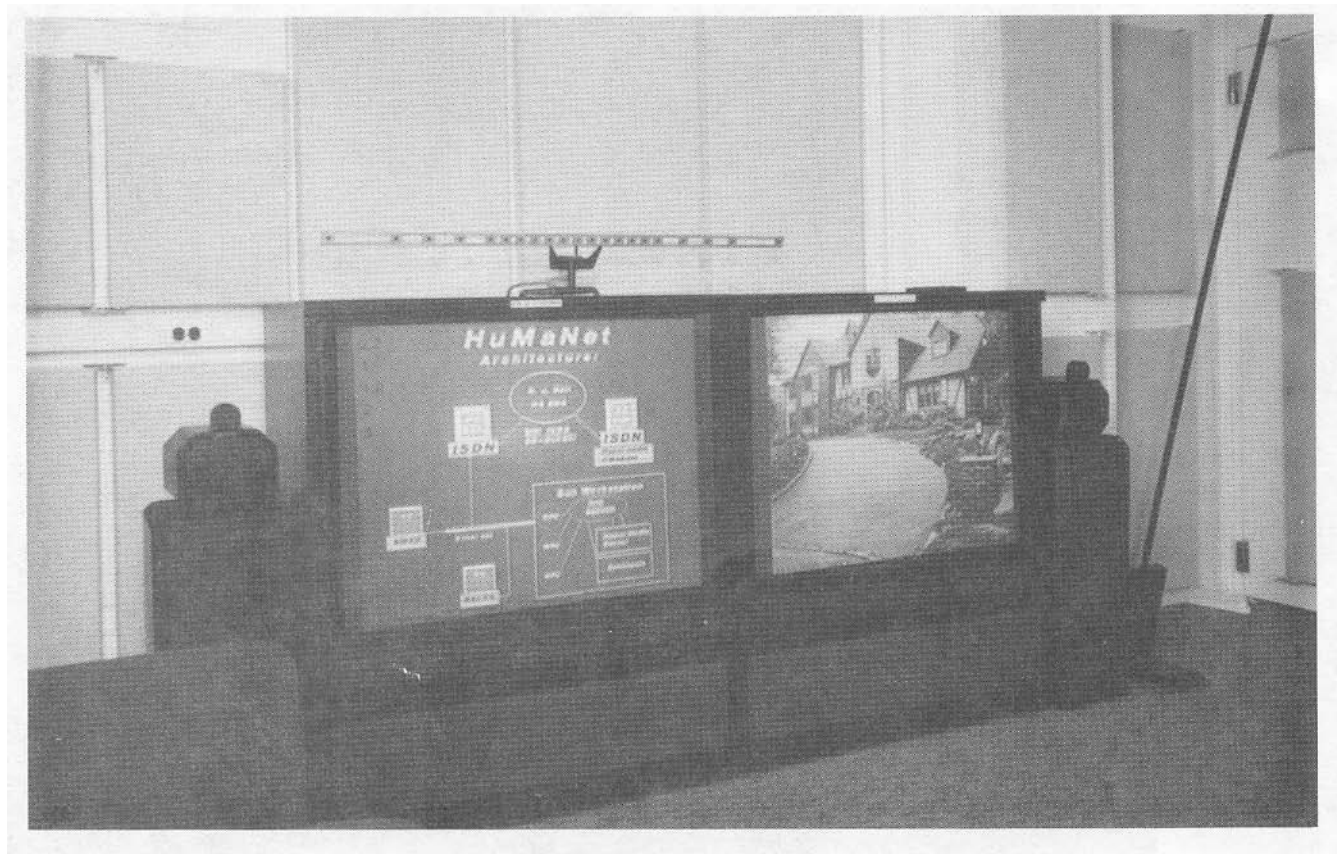
Fig. 3. (a) Auditorium installation of a 2D autodirective array. (b) Teleconferencing application of a 1D autodirective array. The array provides input to a connected-word speech recognizer for controlling system features [4].
