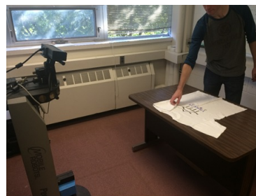
Figure 1: The setting of our situated task learning where a human teacher teaches the robot how to fold a T-shirt through both task demonstrations and language instructions.
