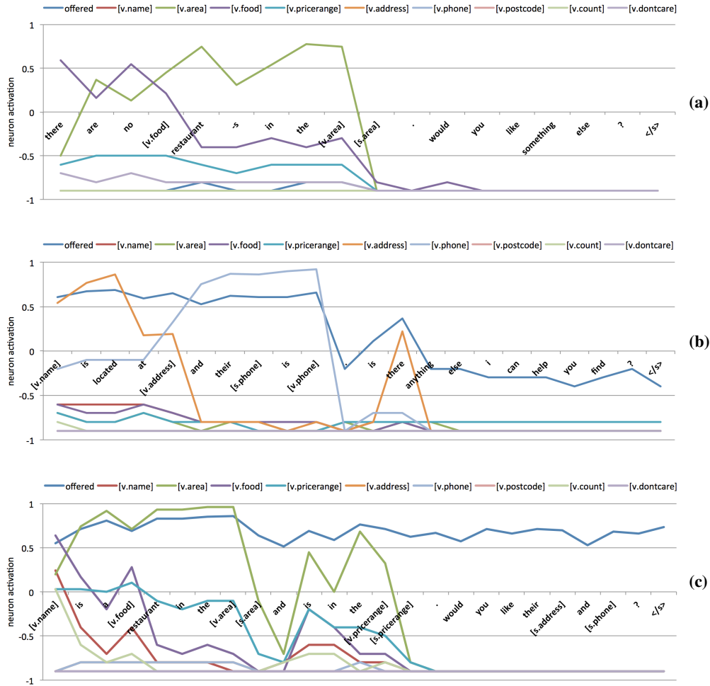
Figure 4: Three example responses generated from the hybrid model trained with snapshot and attention. Each line represents a neuron that detects a particular snapshot event.
