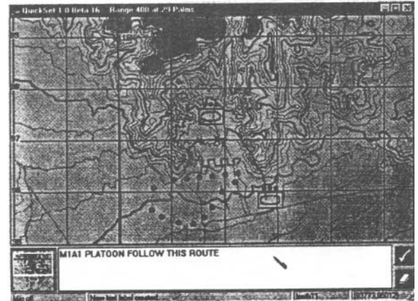
Figure 4: The QuickSet interface as the user establishes two platoons, a barbed-wire fence, a breached minefield, and then issues a command to one platoon to follow a traced route.
