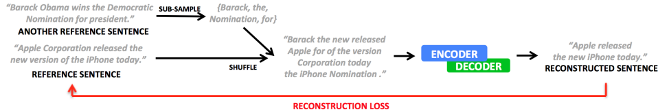
Figure 1: Illustration of Additive Noising. A reference sentence is noised with subsampled words from another sentence, and then shuffled. The denoising auto-encoder is trained to recover the original reference sentence. This simulates a text summarization training regimes without the need for parallel corpora.
