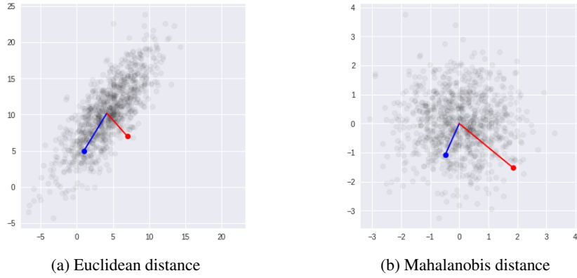
Figure 1: Euclidean distance to the mean in a multivariate normal distribution is not necessarily related to probability; in figure (a), the red vector, despite being an outlier, is closer to the mean. In figure (b), we have rescaled and decorrelated the distribution; Euclidean distance measured in the resulting space (the Mahalanobis distance) can be related to probability through the \chi^2 distribution.
