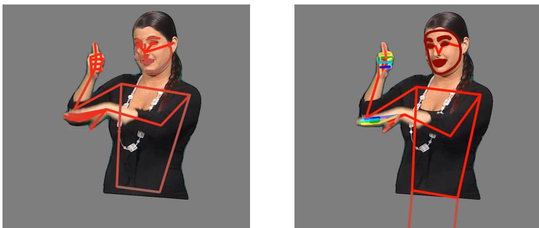
Figure 3: Examples of the output of pose estimation systems overlaid over the original video frames. Left: OpenPose, right: MediaPipe Holistic.
