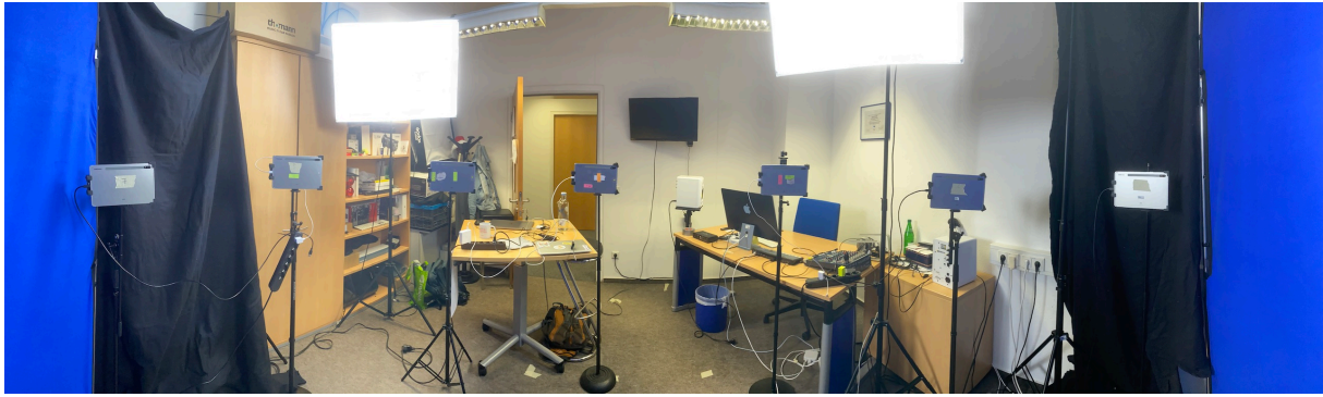
Figure 2: A 180 degrees panoramic view of the recording setup from the point of view from the Signer. The Director sits just behind the frontal camera. The Operator sits at the table next to the Director.
