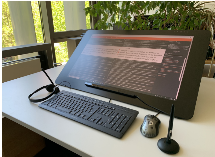
Figure 1: Hardware setup with a large tiltable screen, a digital pen, mouse, keyboard, a headset, and an eye tracker.
