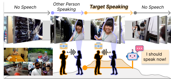
Figure 1: EgoSpeak models speech initiation in real time from the camera wearer’s (camera icon) egocentric video stream, mirroring how a real-world agent would perceive and engage in dynamic, multi-speaker environments.
