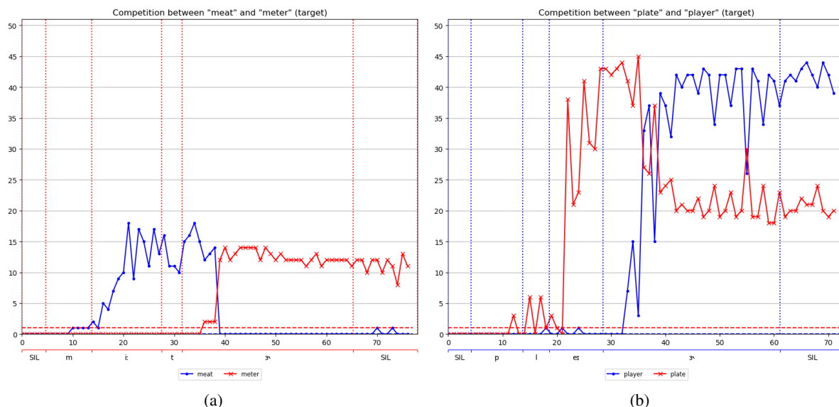
Figure 5: Illustration of lexical competition between 5a “meat” and “meter” (target) and 5b “plate” and “player” (target). Numbers in 1 st x-axis corresponds to the number of MFCC frames; 2 nd x-axis corresponds to time-aligned phonemic transcription of the target word; y-axis shows number of images for which at least one caption (out of 5) contains the target or competitor word. Vertical colour bars are projection of phoneme boundaries of the target word. Horizontal colour bars show chance score for each word (<2).
