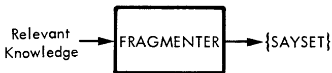
Figure 5. Fragmenter module input and output.
