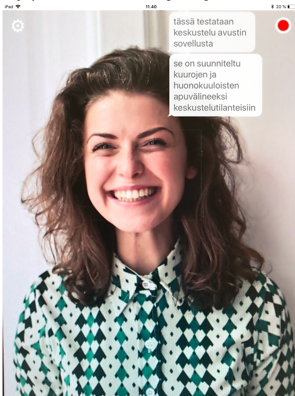
(b) Mobile AR version. The speech recognition results are placed in speech bubbles next to the face of the speaker.
