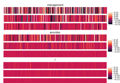
Figure 1: Visualization of values in LSTM hidden layers for a noun (top), verb (middle) and question mark (bottom). Each heatmap shows the 256 values returned by each layer, in 3 layers for each word.
