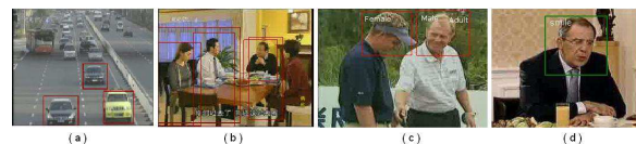
Figure 9: Image processing can be erroneous: (a) only three cars are identified although there are many vehicles prominent, (b) five persons (in red rectangles) are detected although four are present; (c) one male is identified correctly, other male is identified as 'female'; (d) detected emotion is 'smiling' though he shows a serious face.
