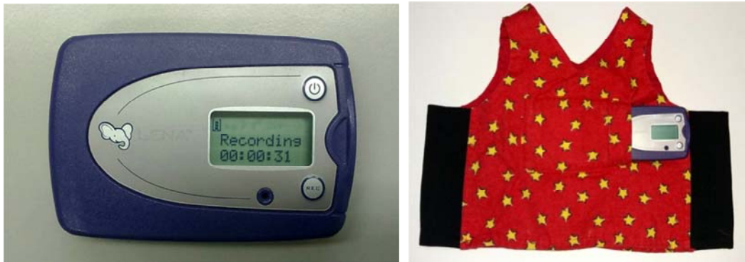
Figure 1. The LENA digital language processor (DLP) placed in the pocket of a vest
