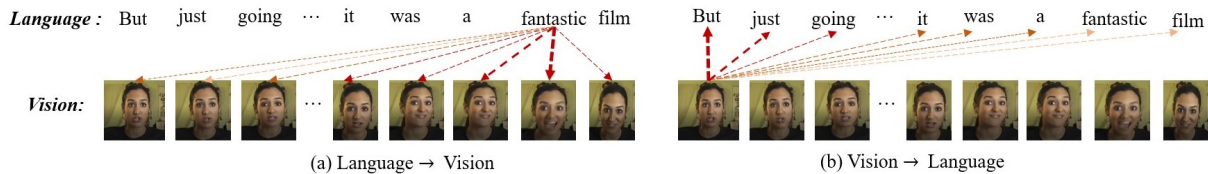
Figure 1: Contexts of each modality captured by crossmodal coattention. (a) shows each language temporal captures context of vision modality by different attention weights. (b) shows each vision temporal captures context of language modality by different attention weights.
