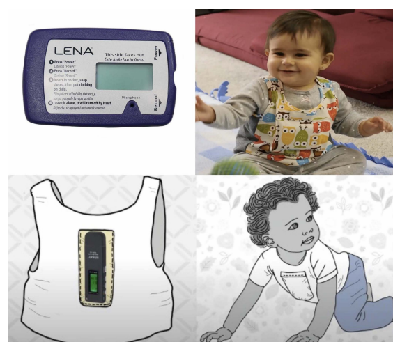
Figure 1: Top: LENA recording device placed in a child’s vest (from Listen and Talk); Bottom: a USB recording device placed in the pocket of a child’s shirt (from videos produced by the LAAC team)
