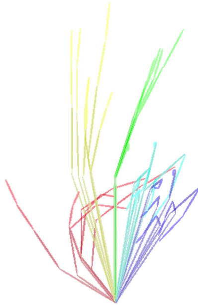
Figure 12: Normalized hand poses overlaid after being translated to the same position. The positions of the wrist and the metacarpal bone of the middle finger are fixed.
