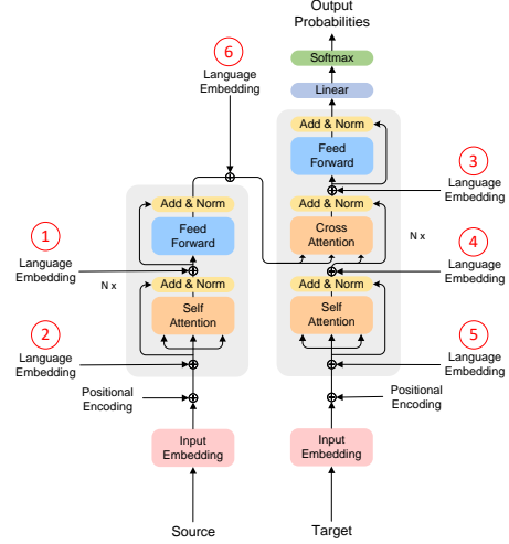
Figure 1: Illustration of the language embedding embodiment strategy. Six switching points in the standard Transformer are particularly marked to insert the language embedding.
