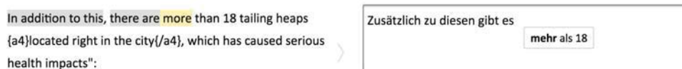
Figure 1: Interactive translation prediction in CASMACAT: The system suggests to continue the translation with the words mehr als 18 , which the user can accept by pressing the TAB key.
