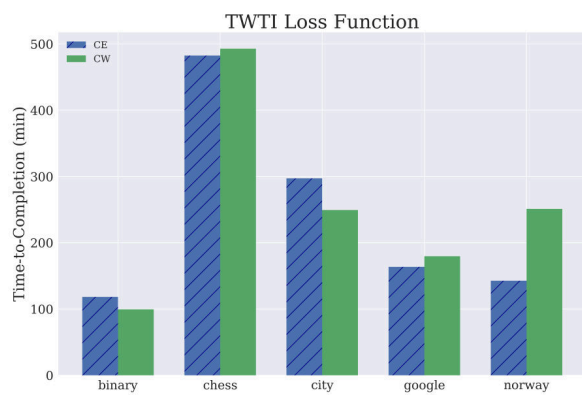
Figure 10: Using the Carlini-Wagner loss function did not significantly improve optimization time-to-completion over standard cross-entropy loss.
