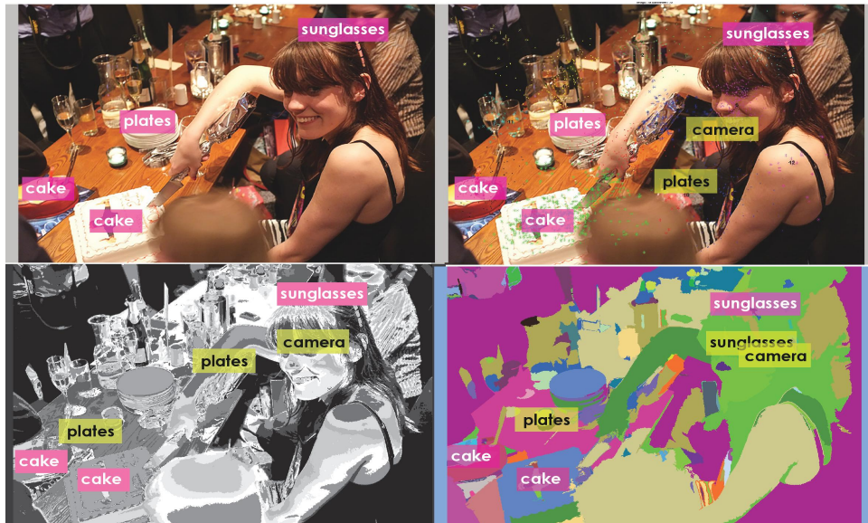
Figure 5: Example region annotations. Top-left: Reference alignments. Alignment output using: top-right: MSFC; bottom-left: modified k -means; and bottom-right: GSEG. Correct alignments in pink. Misalignments and labels not belonging to reference alignments in yellow.
