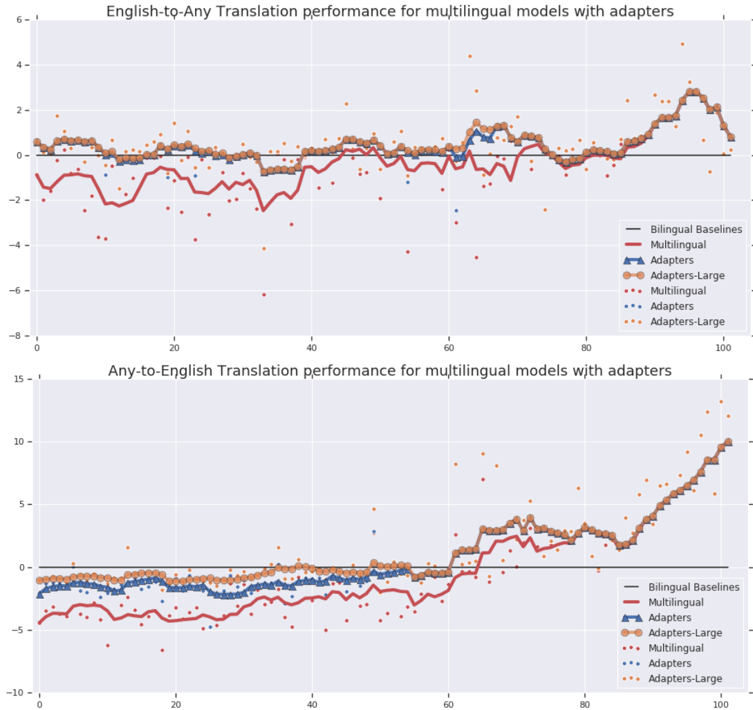
Figure 7: Trendlines depicting translation performance improvement in multilingual models with residual adapters. From left to right, languages are arranged in decreasing order of available training data. y-axis depicts the BLEU score relative to the bilingual baseline trained on the corresponding language pair. The plots correspond to the following models: (1.) Red: Multilingual model trained with sampling temperature, T = 5 (2.) Blue: Multilingual model + Small adapters, b = 2048 (3.) Pink: Multilingual model + Large adapters, b = 4096 . Note: For adapter experiments, we choose the best performance between b = 0 , b = 2048 and b = 4096 .
