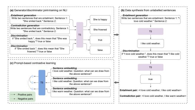
Figure 1: GenSE framework includes three steps: jointly training of generator/discriminator; data synthesis from unlabelled data; prompted-based contrastive learning. All models are initialized from same pre-trained weights. The model with the same colour shares the same weights. The upper-left of each sentence block refers to the prompt name listed in Table 1.
