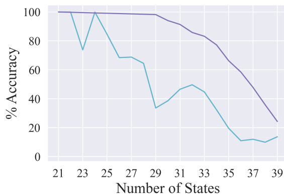
Figure 3: As SFST state size increases, average accuracy (blue line) decreases. Increasing the neural model’s size improves accuracy (purple line).
