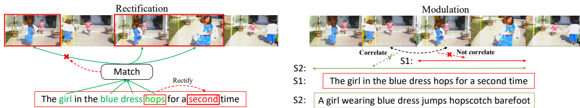
Figure 1: Illustration of rectification and modulation modules for precisely localization. Left: The rectification module helps correct the attention to focus on the best matched position. Right: The modulation module correlates the video contents with different weights referring to different sentence semantics.
