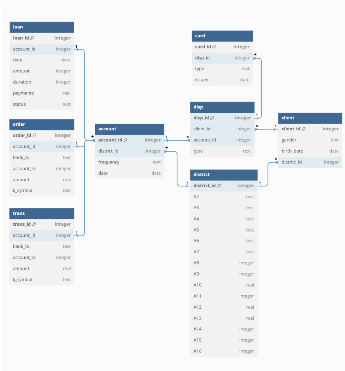
Figure 4: Database schema of the database in the financial domain of BIRD-Bench.
