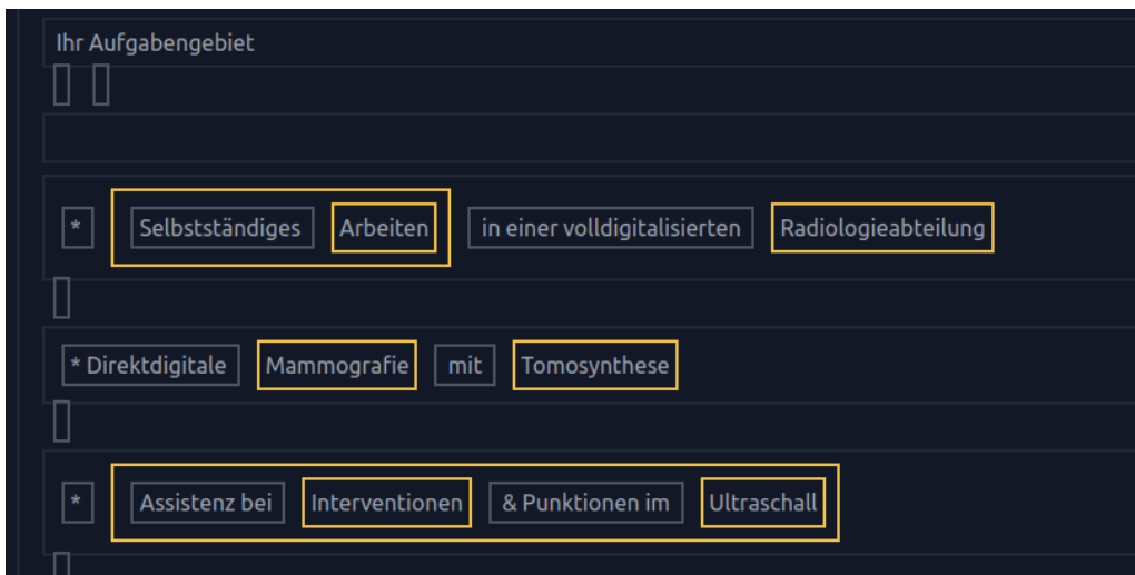
Figure 3: Visualization of the rendered tree structure in Orbis Annotator. The borders were added to illustrate the underlying tree-structure, and are invisible in the Orbis Annotator interface. The border color is used to indicate whether elements are annotated (yellow) or unannotated (grey).
