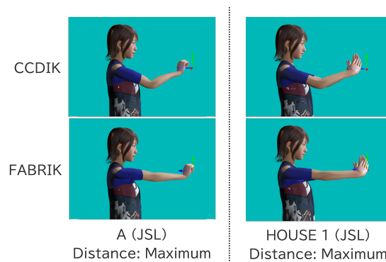
Figure 6: Comparison of IK solvers: CCDIK (upper) and FABRIK (lower).
