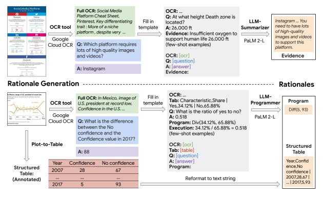
Figure 2: For training examples, we first generate the full OCR of each image with Google Cloud OCR. Depending on the dataset, we either use LLM-Summarizer (few-shot prompted PaLM 2-L) to generate text evidence (top), or use LLM-Programmer (also PaLM 2-L) to generate a program based on both the OCR and available structured table source for the image (bottom).
