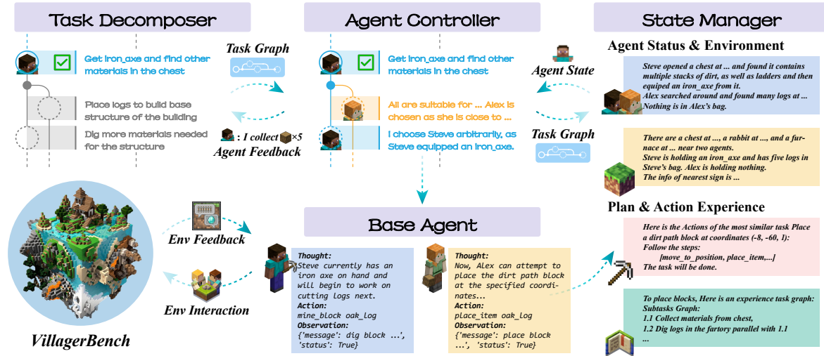
Figure 2: Overview of the VillagerAgent framework. Our framework acts as the central architecture for individual agents, enhancing their collaborative capabilities. Featuring a Task Decomposer that generates subtask DAGs, an Agent Controller for task assignment, a State Manager for status updating, and Base Agents for task execution and self-assessment.
