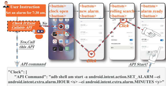
Figure 1: For the task of “Setting an alarm for seven thirty.”, accomplishing it solely through UI operations requires four steps, while API calls can achieve the same task in just one step.
