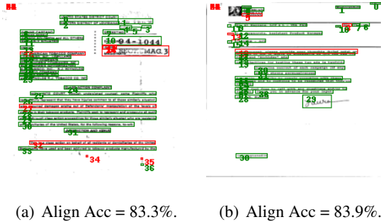
Figure 4: Visualization of learned textline-region alignment. The green and red textline bounding boxes denote the correct and incorrect alignment, respectively.
