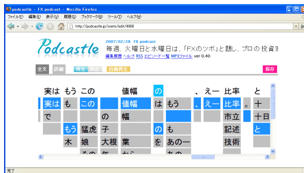
Figure 2: PodCastle screen snapshot of an interface for correcting speech recognition errors (competitive candidates are presented underneath the normal recognition results). Five errors in this excerpt were corrected by selecting from the candidates. The corrected Japanese sentence means “... well, actually the ratio of this price range and ...”.
