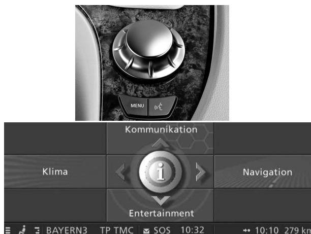
Figure 1: iDrive controller and Central Information Display (CID)
