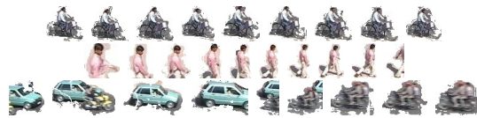
Figure 1: Agents as sequences of isolated foreground blobs. Bottom row (agent 130): the sequence is initially tracking a car - but after it exits, it is erroneously mapped to a motorcycle.
