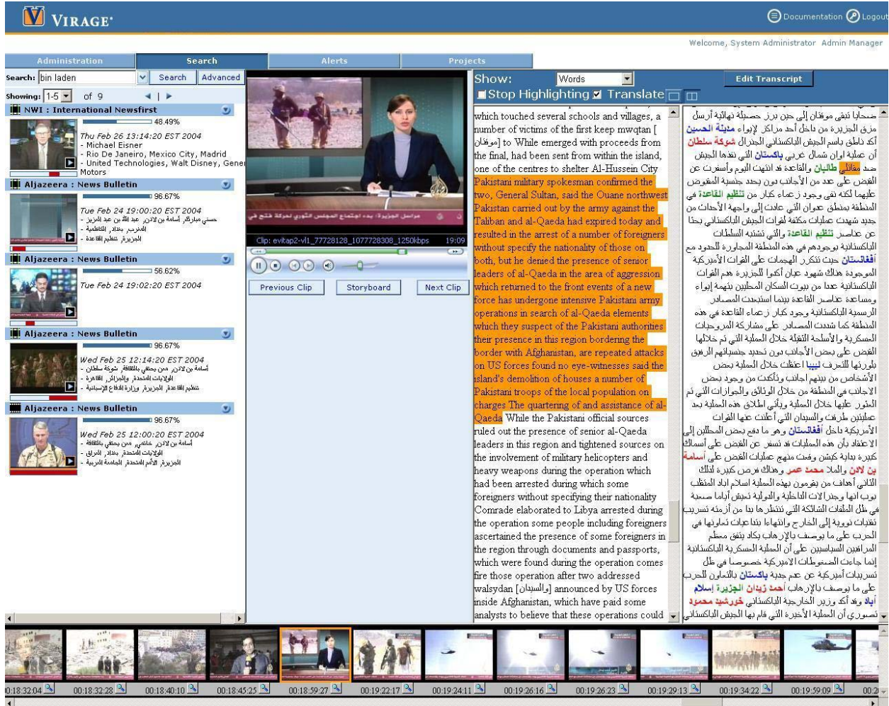
Figure 1: Multilingual alerting and search interface, with alert list, synchronized video playback, Arabic speech recognition output, Arabic-to-English machine translation output.
