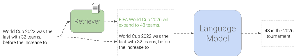
Figure 1: An example of In-Context RALM : We simply prepend the retrieved document before the input prefix.
