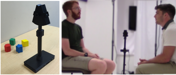
(a) The TreeCam audio/video capture device. (b) Illustration of the task environment. Participants and confederates sat face-to-face while engaging in a “get to know each other” dialogue, with the TreeCam placed in between.
