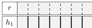
Figure 9: Maximal segmentation where h_1 is the worst possible candidate segmentation relative to the reference r ; at every possible boundary position, it makes the opposite decision.
