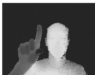
Figure 3: A depth image representing distance from the camera for every point in the human figure (bright points are more distant)
