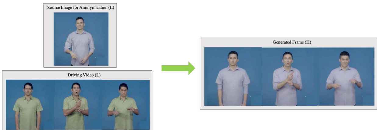
Figure 5: Method Overview: Phase II - Inference. In the inference phase, the source image for anonymization and the extracted frames from the driving video are input to the model. All the images are of low resolution. The model predicts the optical flow and confidence map between the source image and each frame in the driving video. The encoder-decoder takes the source image as input and outputs the high-resolution generated frames with the help of the estimated optical flow and confidence map.
