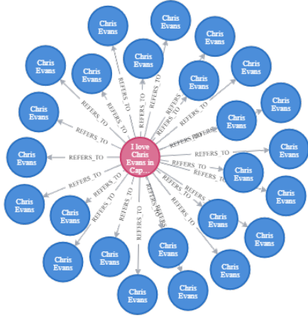
Figure 5: Graph showing how an UTTERANCE node (in pink) can be related to more than one PERSON nodes (in blue) having the same string label (i.e., Chris Evans ). Such cases can be disambiguated through the PageRank algorithm.
